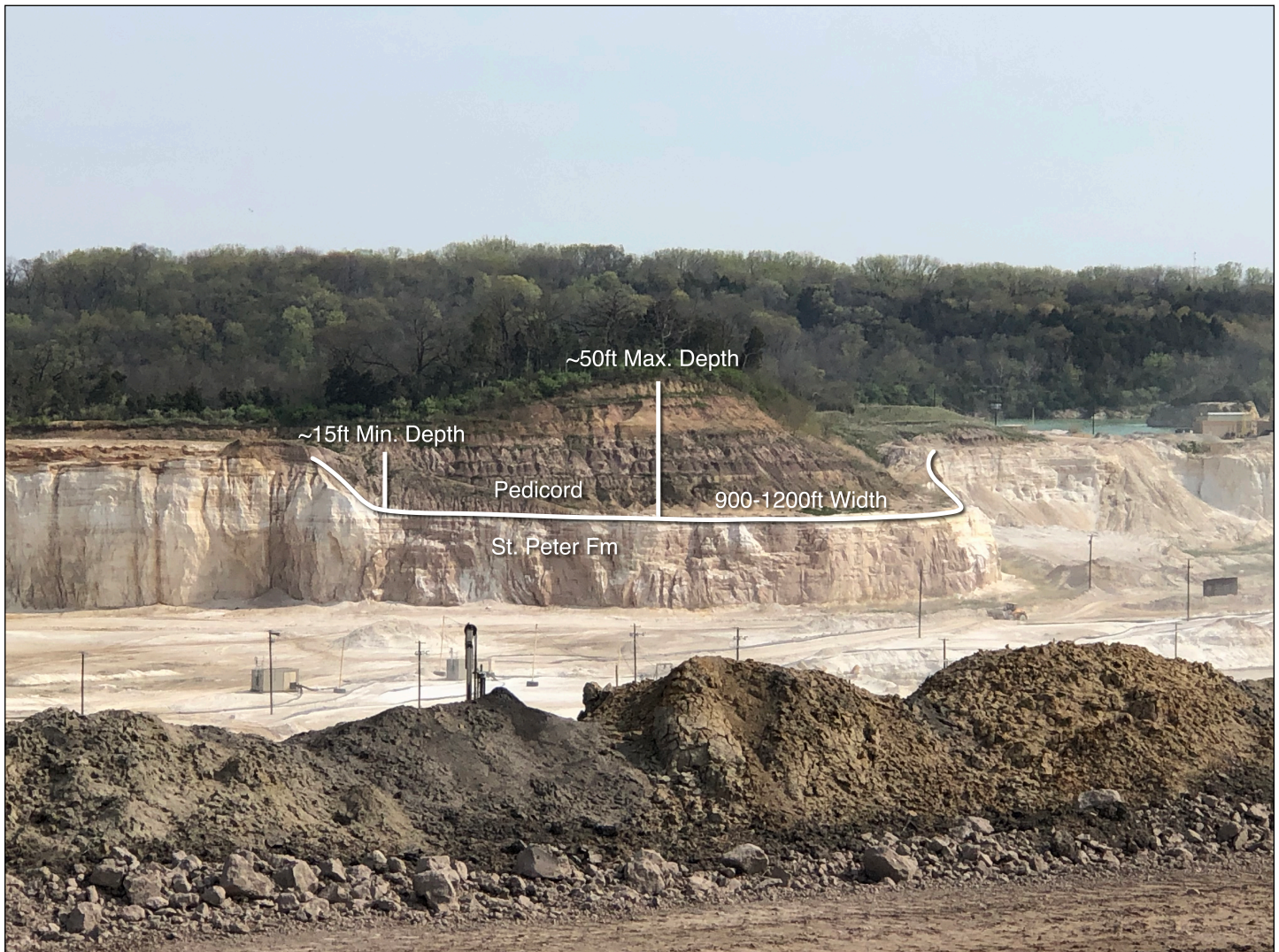
Photo 5 Showing the preglacial valley fill of the Ticona River in the Wedron Silica Pit, photo looking north. Location is field note W17 which is shown on the quadrangle map accompanying this report.
