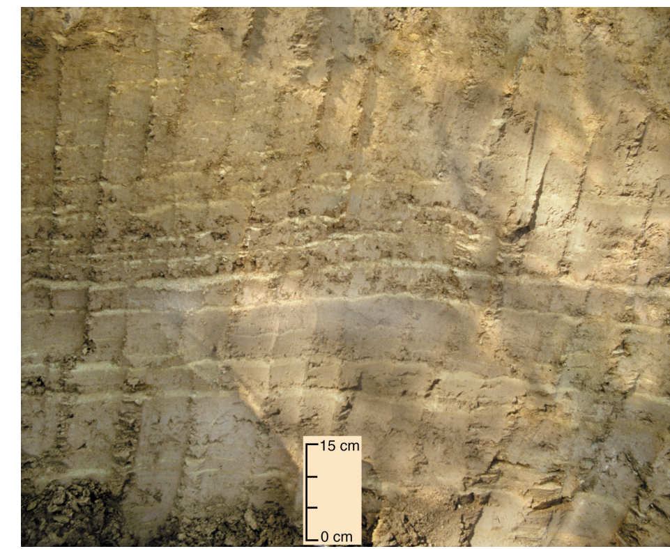
Figure 4 A closeup of laminated lake sediment (Equality Formation) at exposure site 16f (SE, NE, NW, Sec. 27, T42N, R7E). The sediment consists of silt loam (thicker beds) interlaminated with very fine sand. Laminations occur rhythmically every inch or two and probably represent seasonal or diurnal variations in glacial discharge energy.
