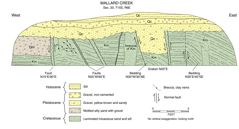
Figure 1 Sketch of north bank of Mallard Creek showing fault zone (modified from Nelson et al. 1999).
