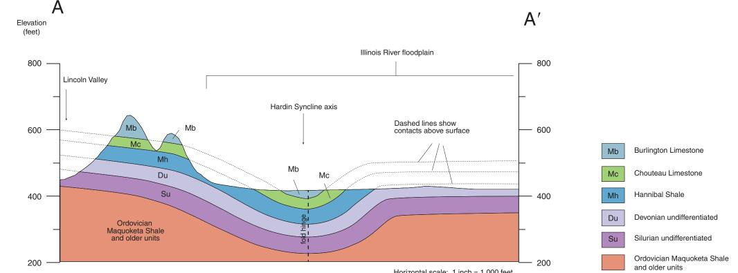
Horizontal scale: 1 inch = 1,000 fee Vertical scale: 1 inch = 200 feet Vertical exaggeration: 5x Quaternary deposits not shown
