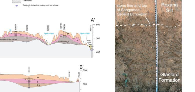
Figure 4. Contact between the Roxana Silt and the Glasford Formation. The contact is often distinguished by a thin layer of pebbles ("stone line") that was formed during development of the Sangamon Geosol. The staff gauge is marked in feet.
