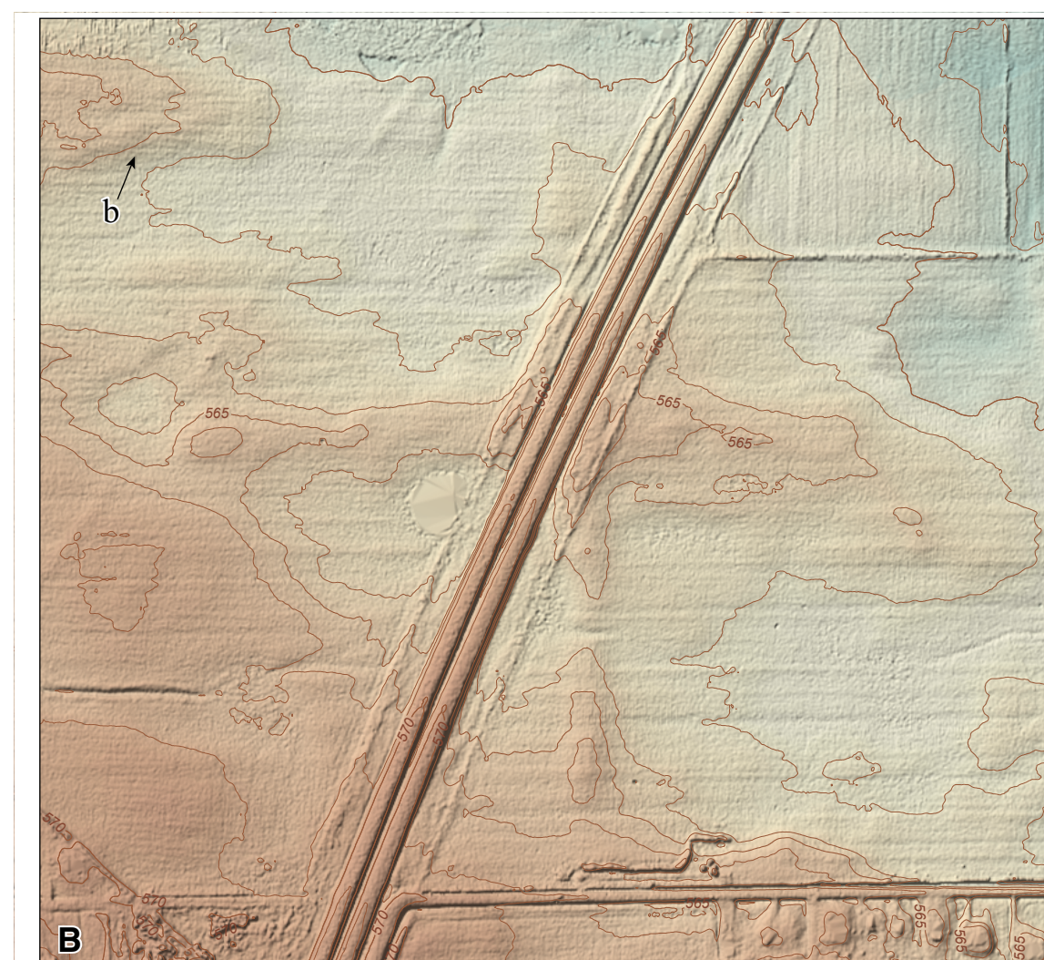
Figure 3 The feature shown is a cloverleaf interchange structure associated with I-55 located at the Will County boundary (T32N, R09E). Figure 3A is a digital surface model (DSM), whereas Figure 3B is a DTM of the same area. In contrast to a DTM, which represents only ground features, a DSM portrays all aboveground features. For example, the roadway overpass (a) shown on the DSM has been removed on the DTM because the elevated roadway is not considered part of the ground surface. Likewise, the patterns of scattered points at (b) on the DSM represent the cables of an aboveground transmission line, which have been removed on the DTM. Vehicles moving along I-55 (c), building structures (d), and trees and other vegetation (e), all of which are visible on the DSM, have been removed on the DTM. Scale is 1:6,000 (1 in. = 500 ft).
