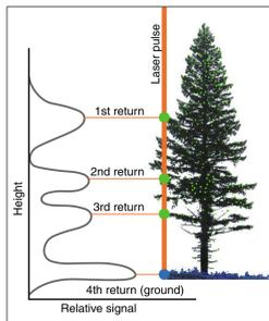
**Figure 1** Simplified illustration of a single laser pulse interacting with a soft target (the tree). A maximum of four returns are possible from each pulse, and current airborne systems can emit more than 150,000 pulses per second. The waveform data collected from the target are processed into a LIDAR point cloud (colored dots), which is used to generate a three-dimensional representation of the target (revised from Mangold and Van Sickle 2008).
