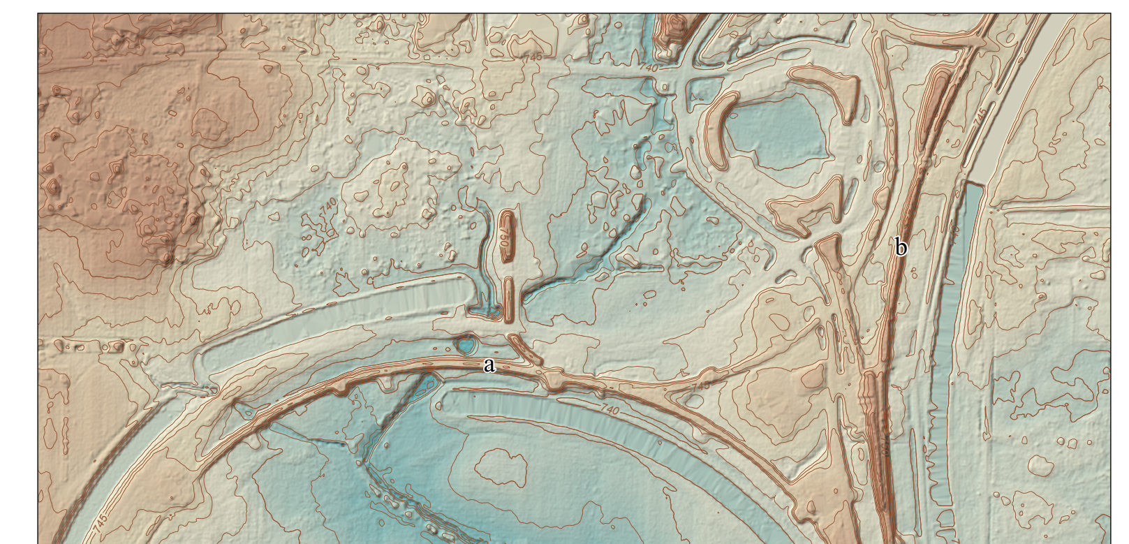
Figure 2 LIDAR digital terrain model (DTM) of the Fermi National Accelerator Laboratory site (T39N, R9E), showing portions of the two principal circular structures, the smaller Main Injector (a) and larger Tevatron (b). A DTM represents only the ground surface and is extracted from airborne LIDAR data using automated filtering methods to produce what is commonly referred to as a "bare-earth" point cloud. Contours are shown at 2- and 5-foot intervals. Scale is 1:6,000 (1 in. = 500 ft).
