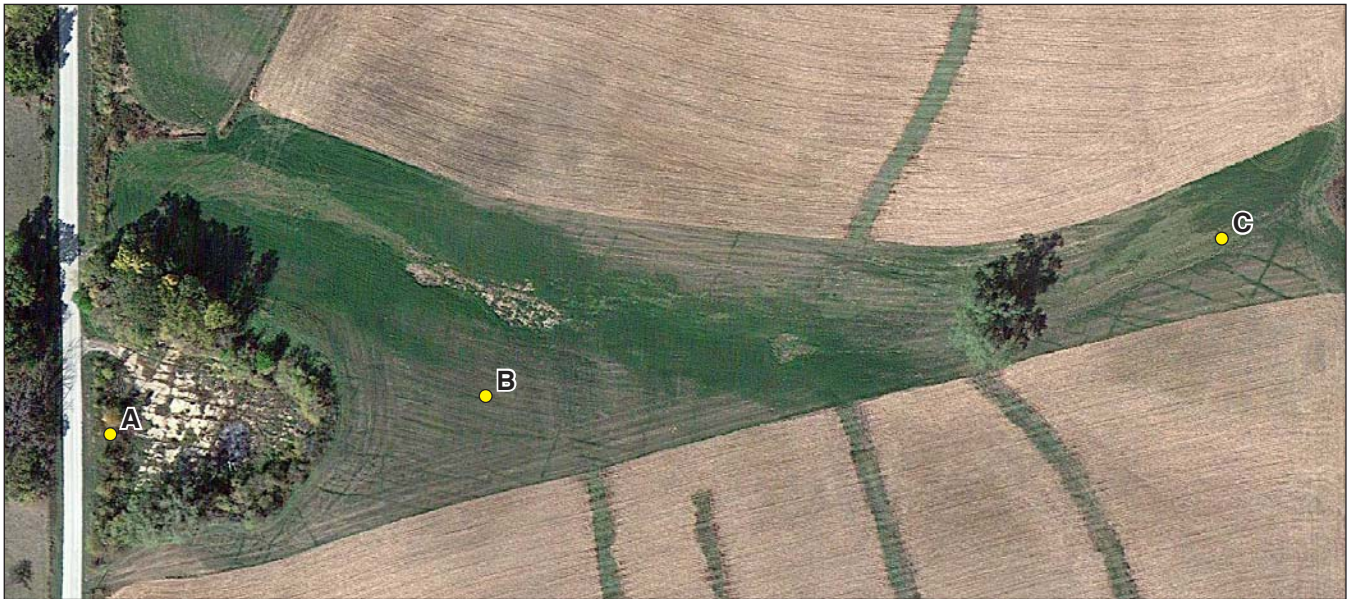
Figure 11 Example of the Google vertical aerial photography acquired on September 27, 2012 (area CL 146; Map 1 T29N, R2E; see Figure A2 and Table A2). The aerial photograph shows a small abandoned quarry at (A) with exposed bedrock fractures and crevices on the quarry floor. Their orientations correspond to the vegetated crop lines visible at (B) and (C), and are direct evidence that the vegetated crop lines are an accurate reflection of the subsurface bedrock fractures and crevices. North is at the top of the photograph. Scale 1 in. = 205 ft (approximate).
