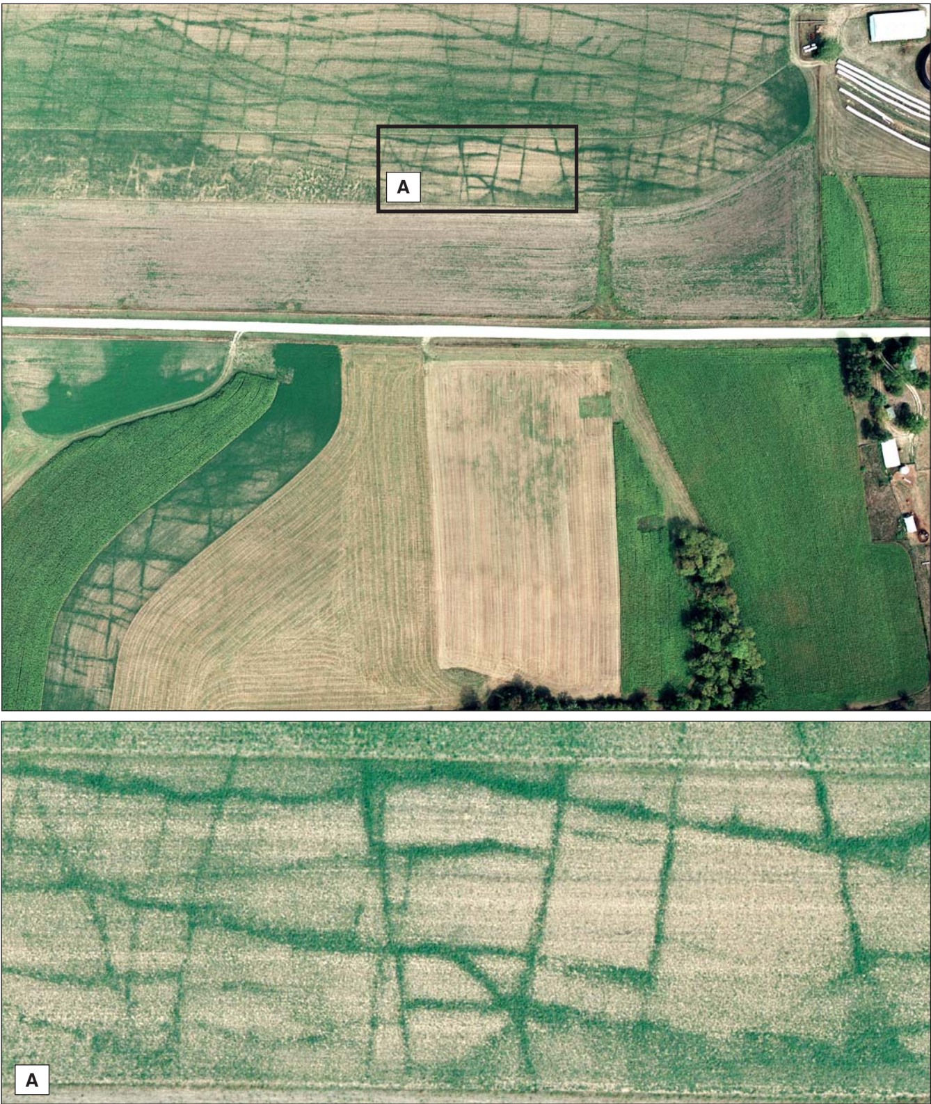
Figure 7 Example of the reconnaissance vertical aerial photography of two alfalfa fields exhibiting pronounced vegetated crop lines acquired on August 28, 2012 (areas ST 10 and CL 48–49; Map 1 T28N, R3–4E; see Figures A1–A2 and Tables A1–A2, respectively). An enlargement of a small portion of the upper field (A) shows in exceptional detail how the alfalfa plants mimic the underlying bedrock fracture and crevice patterns. The more prominent vegetated crop lines shown in (A) average approximately 4 ft (1.2 m) wide, and the varying widths may be indicative of the relative widths of the buried fractures and crevices. North is at the top of the photographs. Scale 1 in. = 250 ft (upper photograph); 1 in. = 50 ft (enlargement). Scales are approximate.
