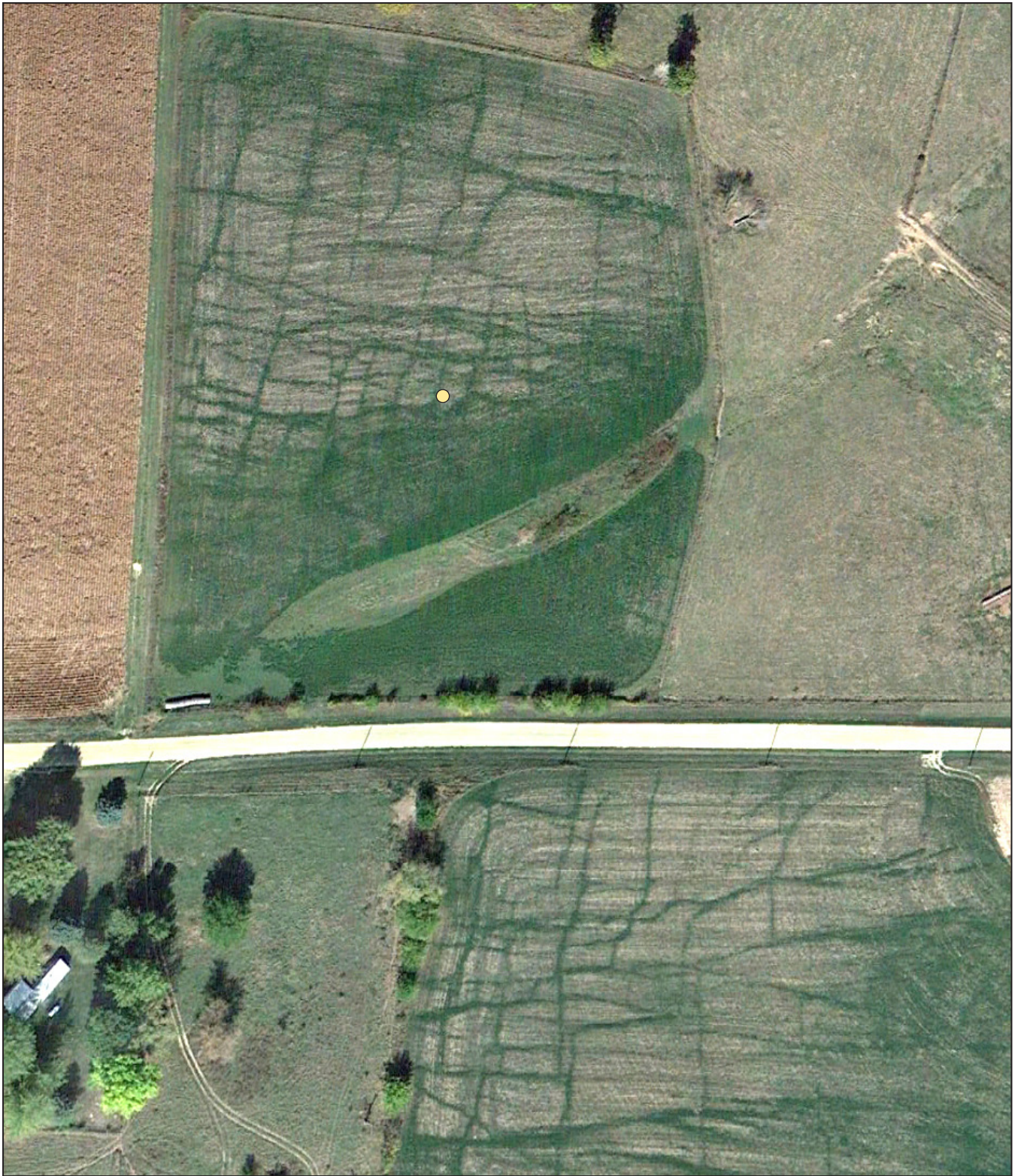
Figure 8 Example of the Google aerial photography of two alfalfa fields exhibiting prominent vegetated crop lines acquired on September 27, 2012 (area CL 24; Map 1 T29N, R4E; see Figure A2 and Table A2). Field excavation in the upper field at the location of the yellow dot revealed a bedrock crevice about 2 in. (5 cm) wide at a depth of approximately 3 ft (1 m), along with an alfalfa tap root embedded in the crevice. The vegetated crop lines visible in this aerial photograph average from 2 to 3 ft (0.6 to 1.0 m) to approximately 6 ft (2 m) in width. North is at the top of the photograph. Scale 1 in. = 115 ft (approximate).
