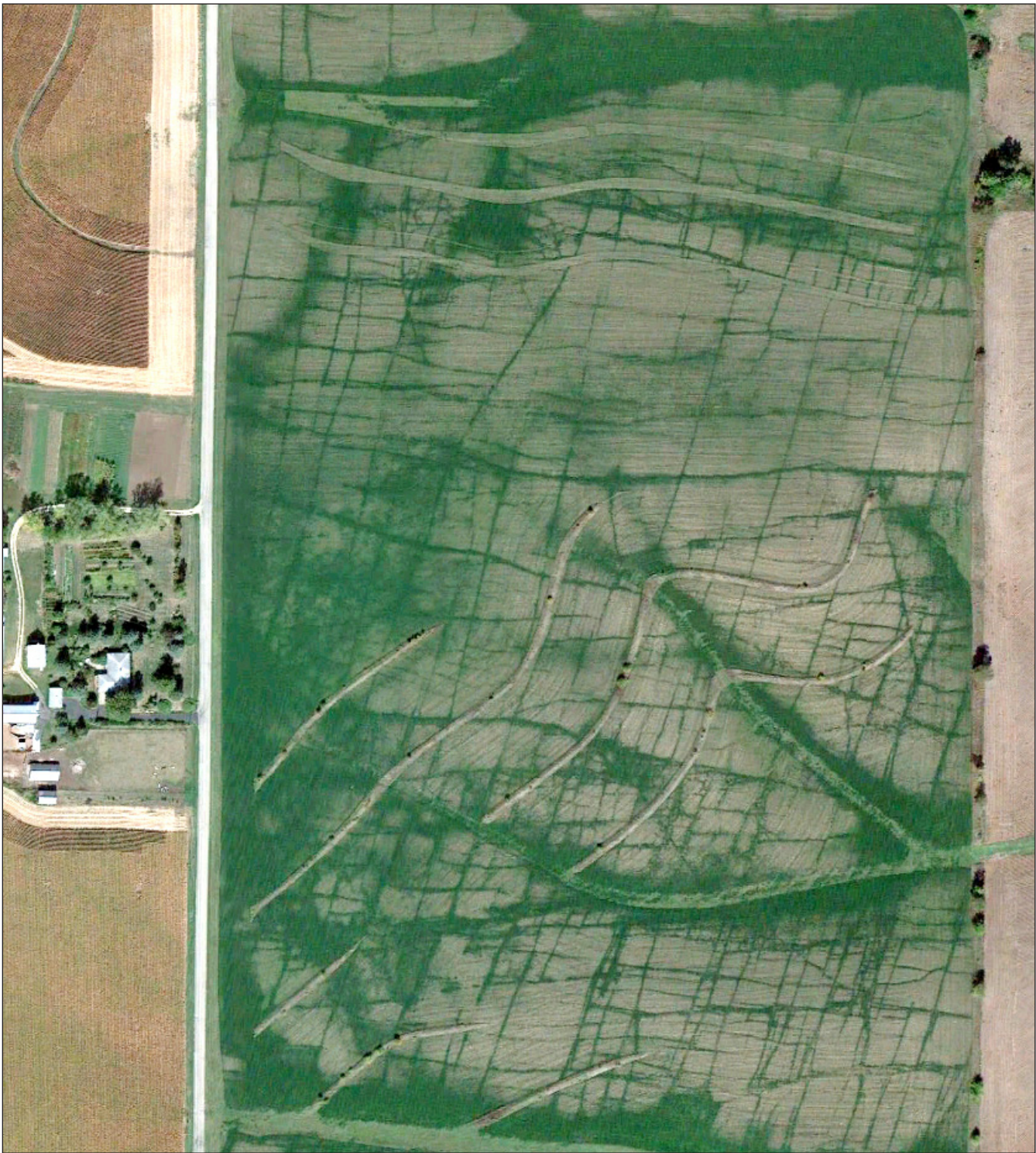
Figure 9 Example of the Google aerial photography of an alfalfa field exhibiting pronounced vegetated crop lines acquired on September 27, 2012. The curvilinear structures within the field are permanent conservation terraces, which are positioned perpendicularly to the prevailing slope to impede erosion. The area is located immediately adjacent to Jo Daviess County in southern Wisconsin (area CL 20; Map 1 T1N, R4E; see Figure A2 and Table A2). The vegetated crop lines visible in this aerial photograph average about 4 to 6 ft (1.2 to 2 m) in width. North is at the top of the photograph. Scale 1 in. = 270 ft (approximate).
