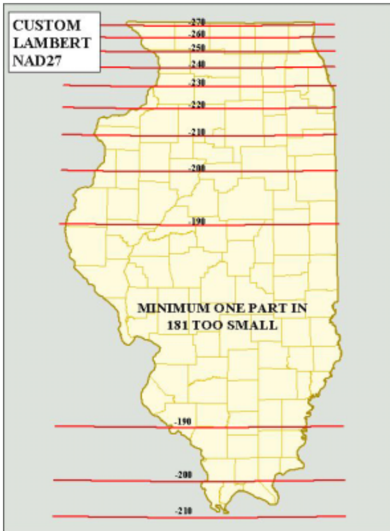
Figure 1. 3 Grid Scale distortions for the Custom Lambert projection (standard parallels 45 North and 33 North)
